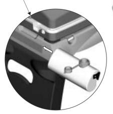
Ignitor on grill bottom fits into slot in plinth.
